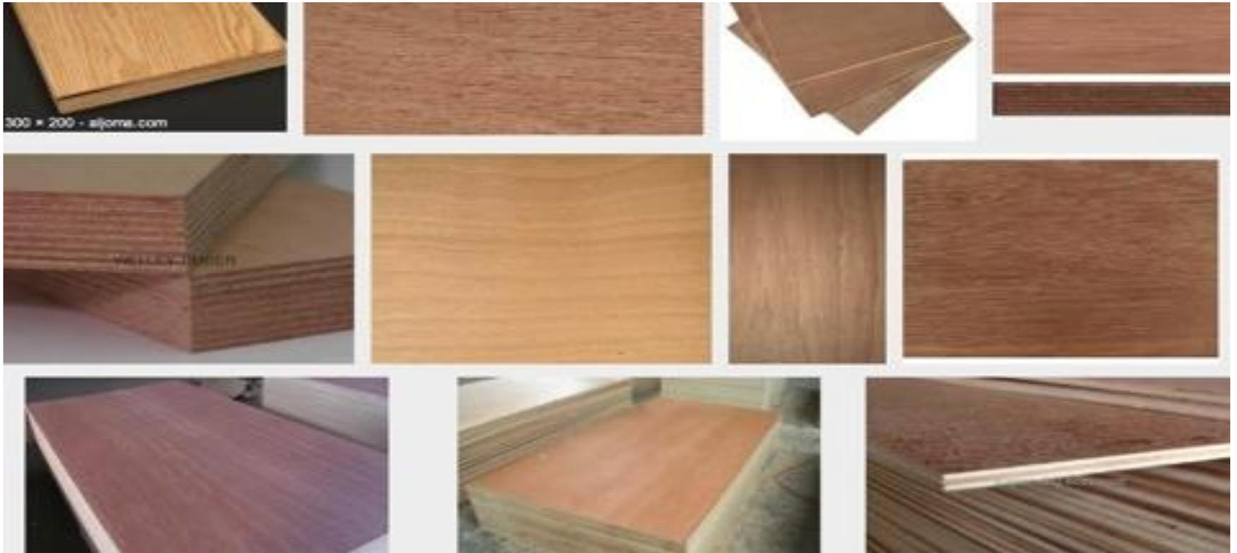
Meranti is used for either plywood, interior furniture, veneer, flooring and construction and boat building.
