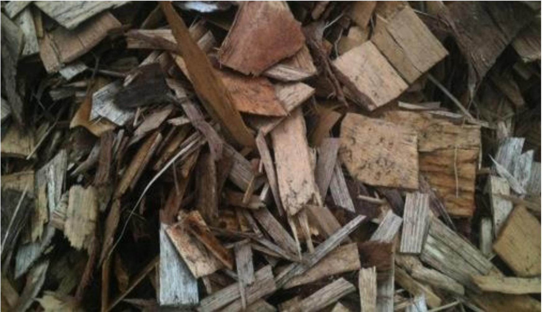
Waste materials from primary and secondary processing are often used as input materials for the production MDF and particle board
