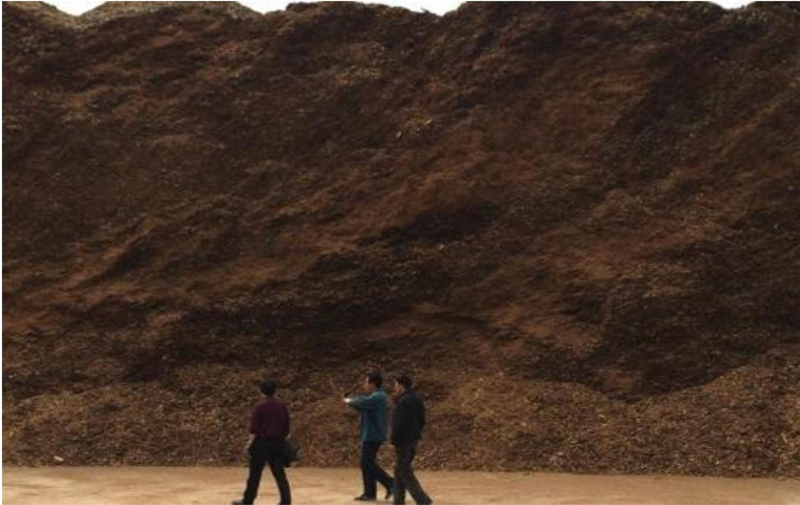
Sawdust (from primary or secondary processing) and wood chips (from waste or forest based materials) for MDF/PB production
